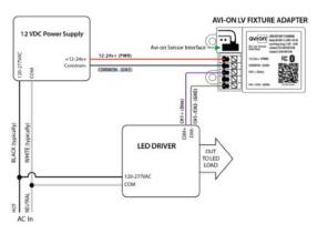
Fixture Adapter connected to LED driver and using power supply
