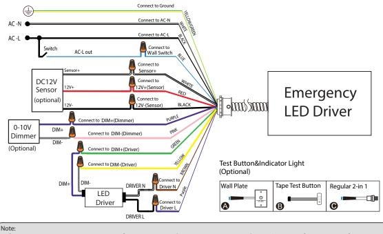
1. If using sensor, sensor wires must remove from LED Driver and reconnect to Emergency driver DC 12V wires for EM Driver to function properly. 2. Cap off if not using dimmer switch
